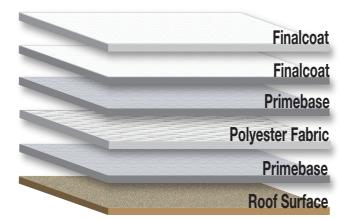
For optimum results seal joints, vents and roof mounted equipment with KM Acrylicaulk. Existing roofs require detailed analysis to determine the most appropriate layers of protection.
